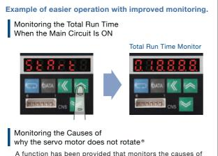
A function has been provided that monitors the causes of why the Servo motor does not move even though a rotation command has been sent.
